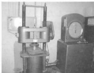
Photo5 Measuring Device of Compressive Strength
