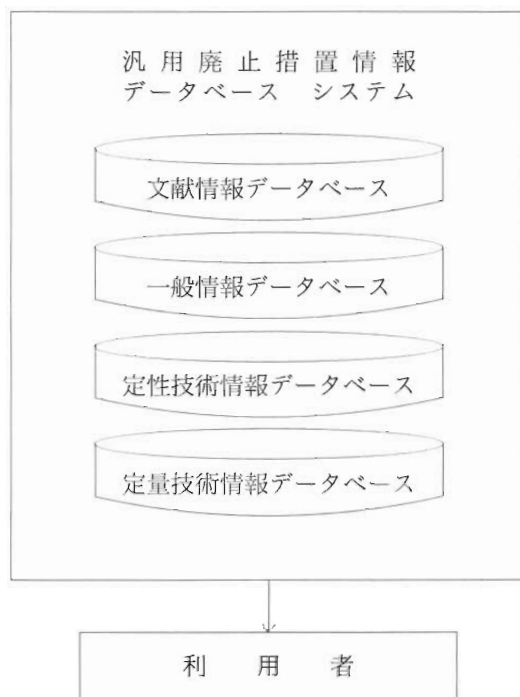
Fig.1 Structure of Decommissioning Database
