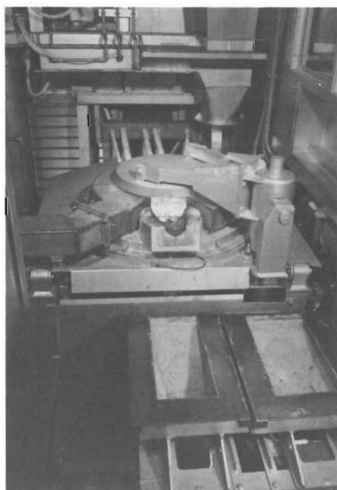
Photo 3 Induction Furnace in JAERI
